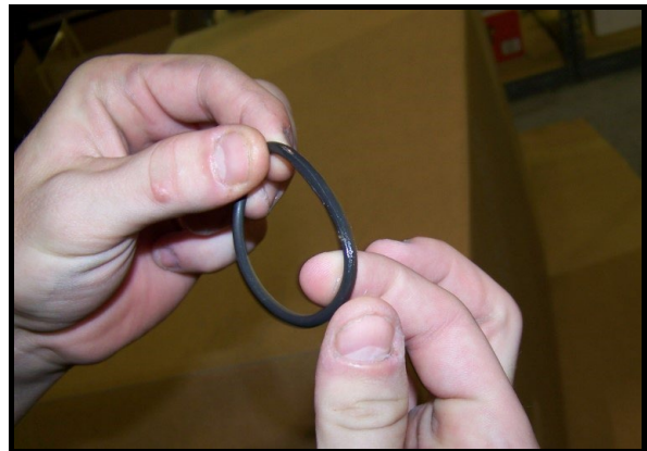
Figure 7 - Lubricating bayonet o-ring.
