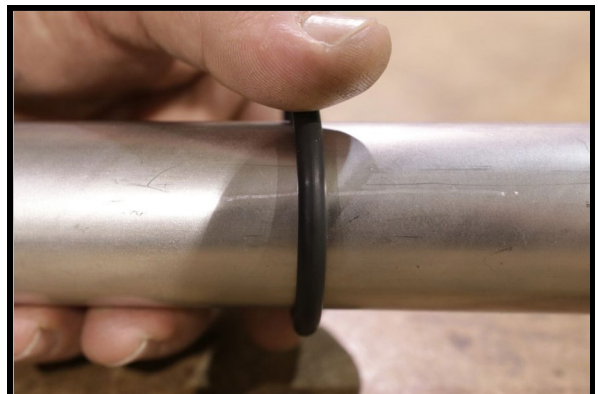
Figure 8 - Installing o-ring on male bayonet.
